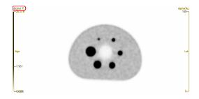
Figure 2.1: Axial slice of the NEMA IEC NM/PET Body Phantom Set<sup>TM</sup>. Red rectangle: data units.
