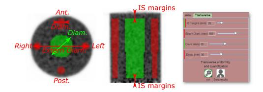
Figure 1.5: Definition of the ROIs for the transverse uniformity test
