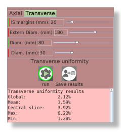
Figure 1.6: Results of the transverse uniformity test
